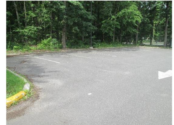
There is an existing vegetated detention basin on site. Parking spaces in the southwest parking lot can be replaced with porous asphalt to infiltrate stormwater and reduce the flow of runoff to the basin. A rain garden can capture, treat, and infiltrate stormwater. A preliminary soil assessment suggests that more soil testing would be required before determining the soil's suitability for green infrastructure.
